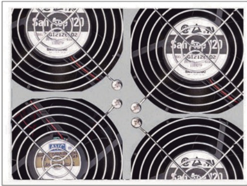
Fan speed controlled by load level
